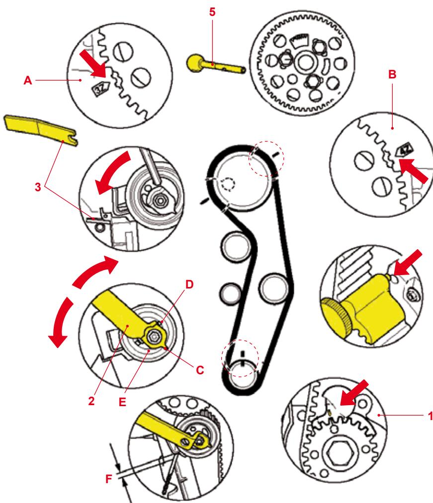
**ENGINES: AJM, ATJ, AVB, AVF, AWX, BDK****Engines 1.9 TDi PD - 2.0 SDi (fig. 2)****Disassembling**
