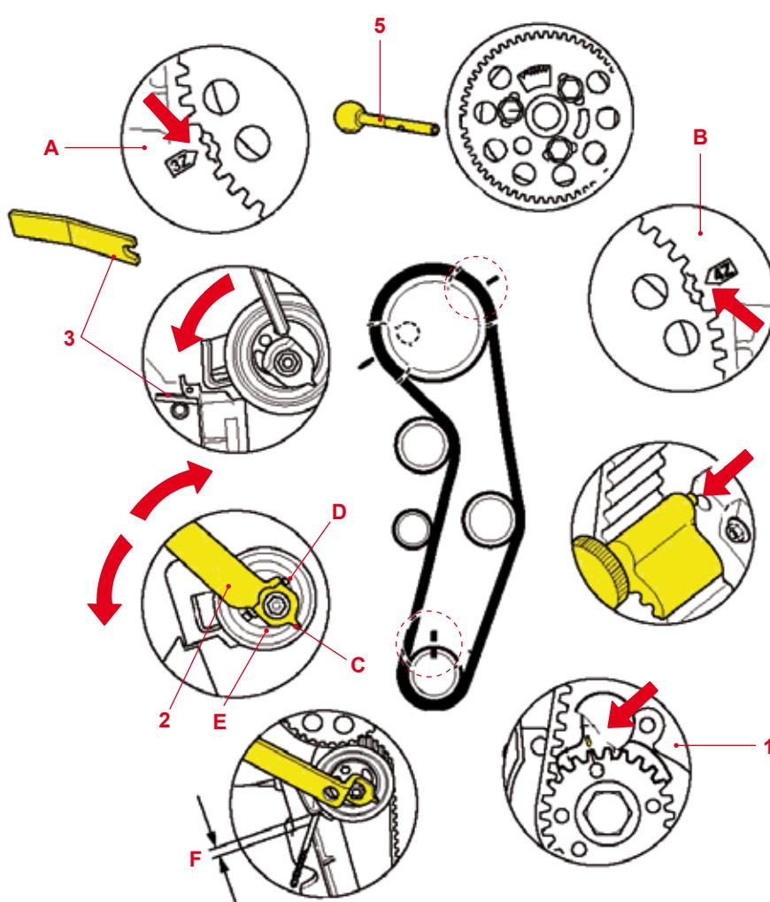
**MOTORES: AJM, ATJ, AVB, AVF, AWX, BDK****Motores 1.9 TDi PD - 2.0 SDi (fig. 2)****Desmontaje**
